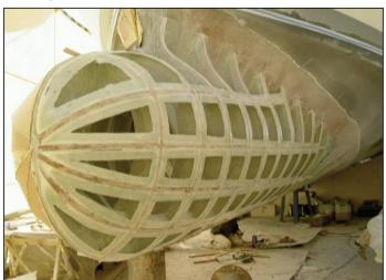
The performance and the speed of the motor yacht were increased with the addition of the composite bulb," stated Bugra Akbiyik, GM, Kompotek A.S.
