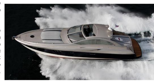
METYX Composites produced custom METYCORE reinforcements for this demanding RTM application. Series production for the elite 55 foot super yacht, which integrates this high-tech hard top, is still going at full speed.
